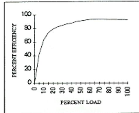
Figure 5.1 Efficiency vs. Loading
