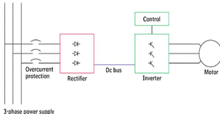
Figure 5.1 Components of a Variable Speed Drive
