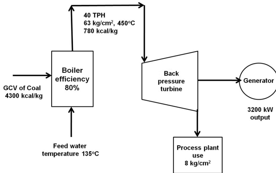
If the steam requirement of the process is to be increased to 44TPH which can be met by the existing boiler through the back pressure turbine,
